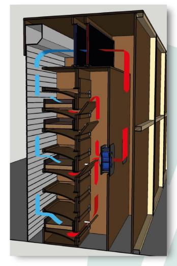
On the left a blowing system: In this version the air is being sucked in at the rear. And is then blown through the seed from bottom to top via a lockable opening. The air is sucked back to the rear through the top.
