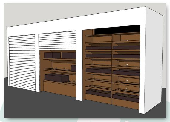
The conditioned drawer or tray dryer is a closed installation. With this installation the seed is dried at the desired air temperature to the desired moisture content. This by using dried and cooled air. The trays or drawers are placed in an air distribution system. Which ensures that the air is blown or sucked through the seed. The air distribution system is located in a closed casing so that the seed can be dried regardless of the outside conditions.
