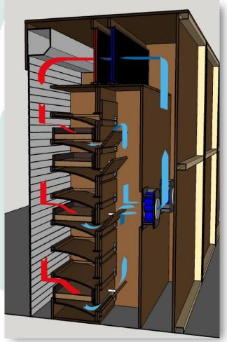
The air is brought to the desired moisture content and temperature at the top of the installation. This ensures that the seed is always dried at the desired air condition. The design of the air treatment installation depends on the required air circulation, the amount of moisture to be drained and the temperature at which there should be dried.
