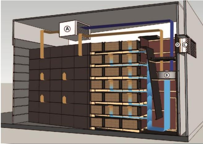
Ventilation system with humidifier and drying option.
