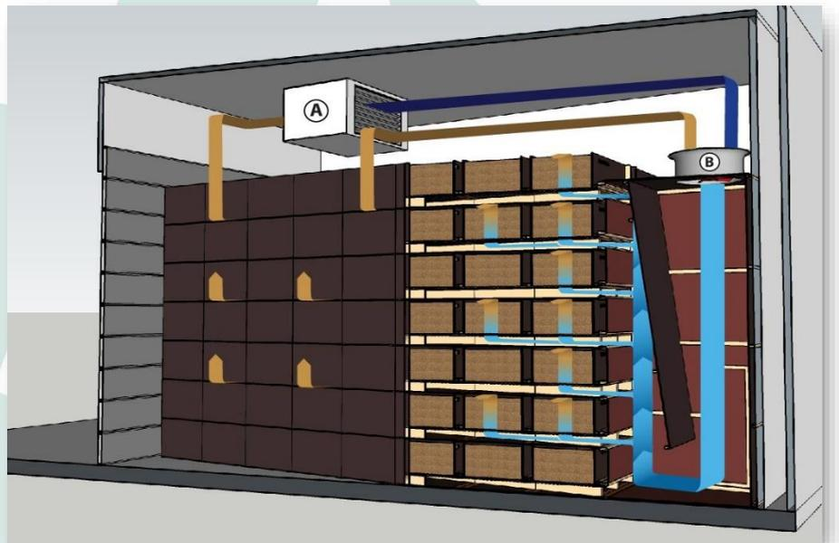
Humidifier in closed cell with internal circulation.
