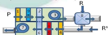
**Option III) 8+9:** Energy saving and reaching any desired T°C for out coming process air. Hybrid system with heat-exchange.
