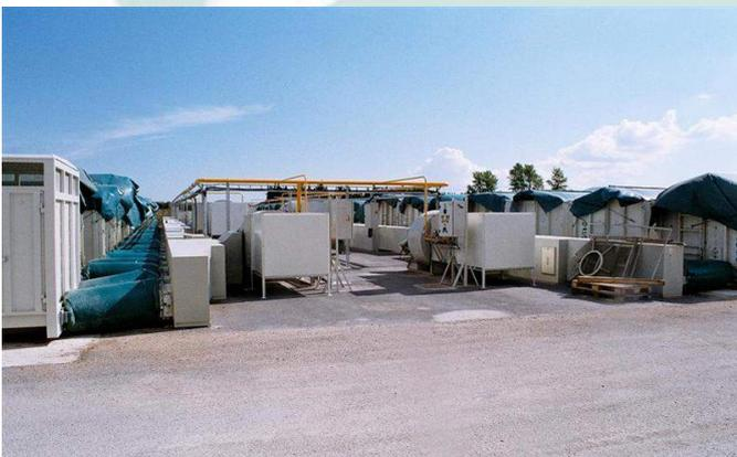
Example of drying process in containers. Airflow would be automatically controlled and on the amount of containers.
