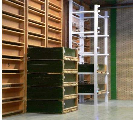
Example of upgrading an existing drying installation with boxes. The boxes with seeds can be dried individually to the required moisture content.
