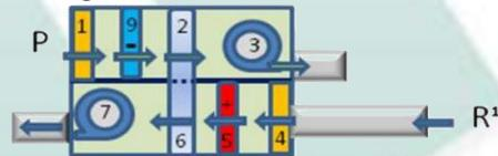
**Option II) 9:** Cold water battery (chiller) with modulated capacity can cool down the process air to any desired T°C. Hybrid system
