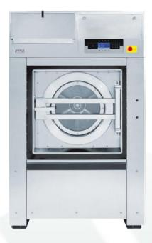
The seed rinsing machine is based on professional or industrial washing machines from the leading brands. These machines are converted, so they will comply with the specifications to be able to professionally clean and treat the seed. On the touchscreen the operator can select the desired recipe or chose an existing recipe. Depending on the user intensity and batch size, the type of machine (professional or industrial) and the capacity (7-180 KG) are selected for you.
