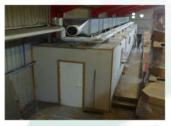
On the right an example of the ABC control for separated boxes; per box and per phase, the desired AH, air quantity and the desired T° are set. This enables the process to pre dry per box with a lot of air and a higher temperature at the start, after which in the last phase the remaining moisture is discharged at a low temperature, with extra dry air and a small air quantity.
