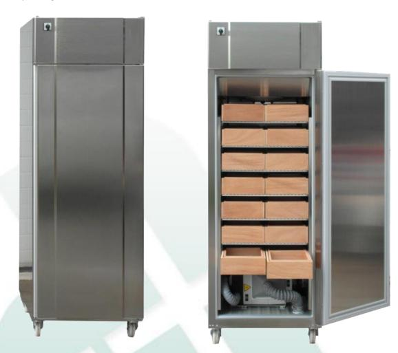
In the static drying cabinet, the seeds are dried and conditioned in bulk in trays or in little bags. The air will blow through the seed in bulk with a light flow (in the trays) or through the baskets with little bags.
