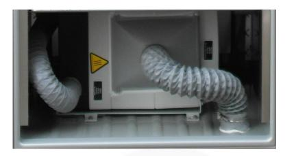
An electrical heating element in combination with a direct expansion cooler will ensure that the desired temperature and moisture content (tot ca 5 gr/kg; 30% RH at 25°C) inside the cabinet is reached and maintained. To gradually reach the low absolute moisture content (1,5 gr/kg; 15% at 15°C), it is possible to also install an adsorption dryer.
