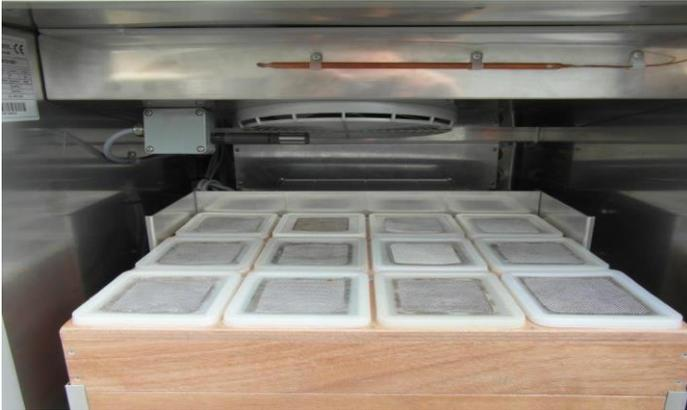
It is possible to configure the air quantity in a pulsating manner. Very vulnerable seeds or pellets will alternate between being in motion and in rest. This way the product will remain loose and aerated without damaging. The product will also dry very evenly.
